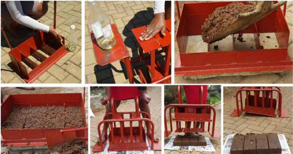
This block maker has been specially adapted to make goat blocks and is available from any hardware shop. (2017 price approx. R1800). Just ask for the HAKA Goat Block maker. If this maker is not available these blocks can be pressed by hand into plastic containers of appropriate size.
